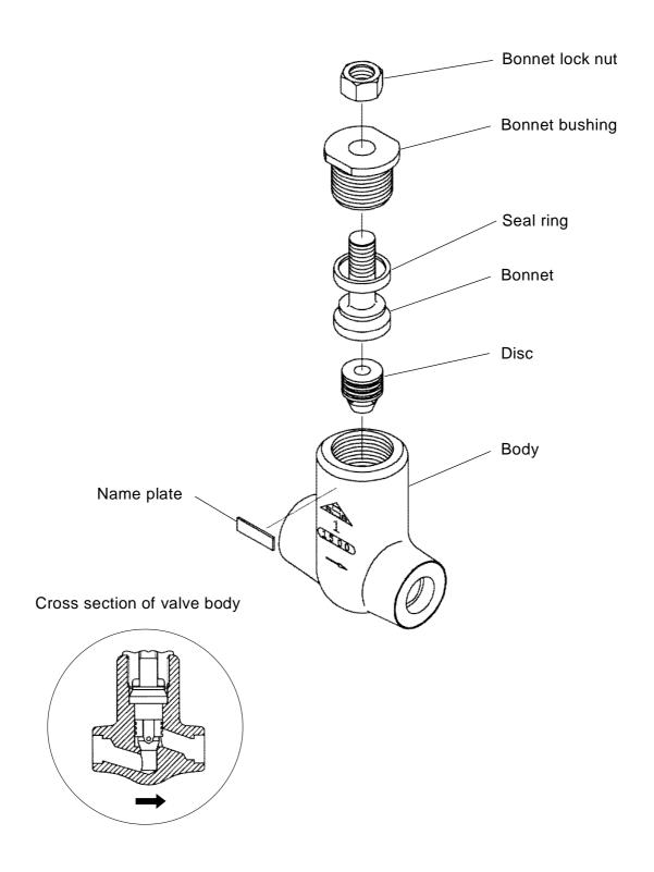
Figure 2.3 Typical Example for Class 1500 Check Valve
