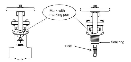
Figure 7.1 Example for Marking Method of Match Mark
