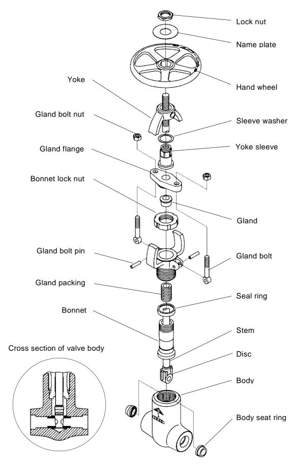
Figure 2.1 Typical Example for Class 1500 Gate Valve
