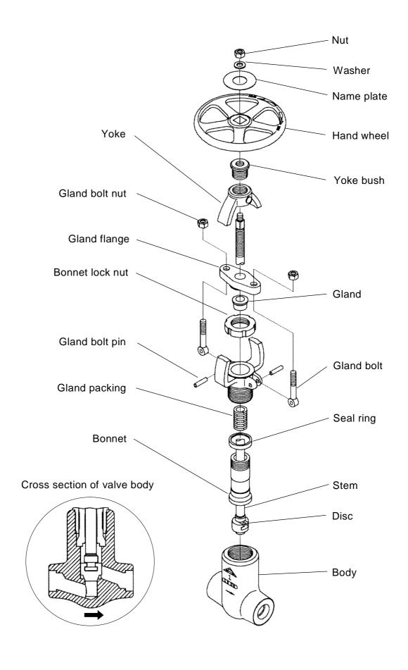
Figure 2.2 Typical Example for Class 1500 Globe Valve
