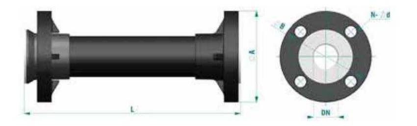
ØA ØB N-Ød DN Ref. JIS ANSI DIN **ANSI** JIS DIN ANSI JIS DIN 20 99 105 70 75 4-16 4-15 300 - 6000 В 108 125 115 79,2 4-16 40 105 110 4-16 4-19 4-18 300 ~ 6000 D 127 140 150 98.5 50 120 125 4-19 155 165 4-18 300 ~ 6000 65 140 145 4-19 178 185 4-18 300 ~ 6000 F 190,5 80 185 200 152.4 150 160 4-19 8-19 8-18 300 ~ 6000 G 100 229 210 220 190.5 175 180 8-19 8-19 8-18 500 ~ 6000 150 285 240 8-23 500 - 6000200 343 340 298.5 295 8-22 12-23 12-23 500 ~ 6000 K 330 290
